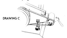
NOTE SLOTTED BRACKET AND LOCKSCREW ADJUSTMENT
