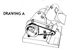
FOR 10,000 RPM NOTE POSITION OF DRIVE BELT ON INNER STEP OF EACH PULLEY
