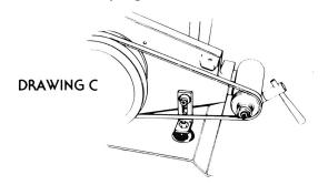
NOTE SLOTTED BRACKET AND LOCKSCREW ADJUSTMENT
