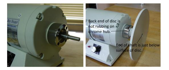
5. Rotate the flat of the shaft so that it is on top or facing up. Slip the disc onto the shaft with the set screw facing up and align it with the flat. Slip it all the way on until the end of the shaft clears or is below the surface of the disc. Make sure that the back end of the disc is not rubbing on the chrome hub. Secure the set screw using a 5/32" hex wrench.
